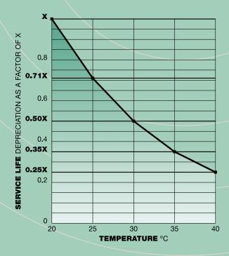
In case of elevated ambient temperature float voltage compensation is recommended. Reference should be made to the Manufacturer's recommendations.
